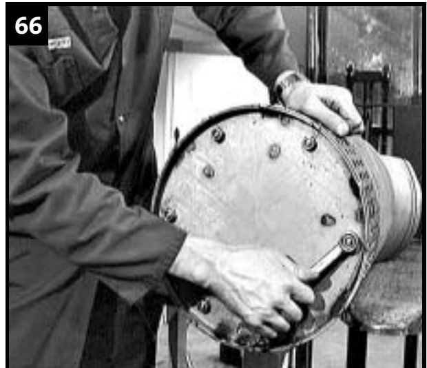
Tighten lock nuts for strainer.
