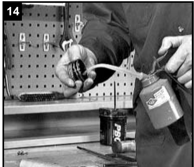
14 Lubricate inside of upper shaft seal.
