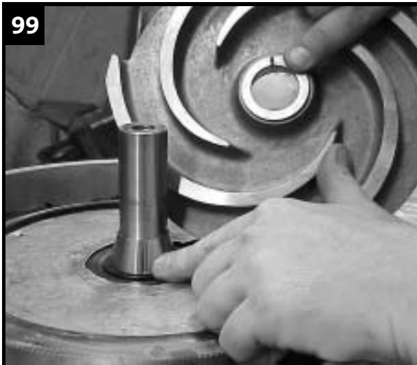
99 Position groove in opposit position.
