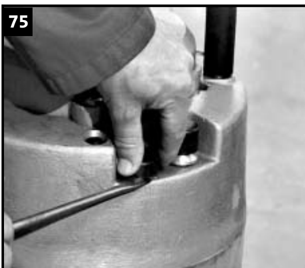
75 Remove rubber cap for level electrodes.
