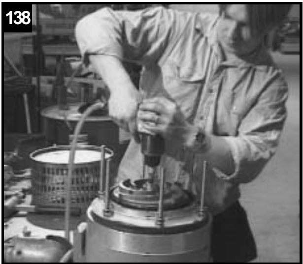
Fit impeller washer and screw and tighten.
