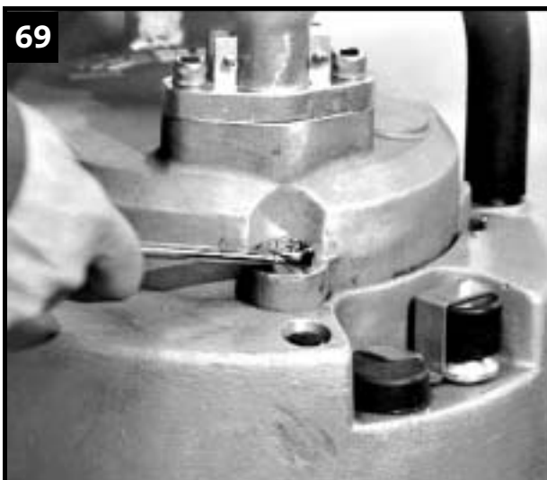
Remove screws in top cover.
