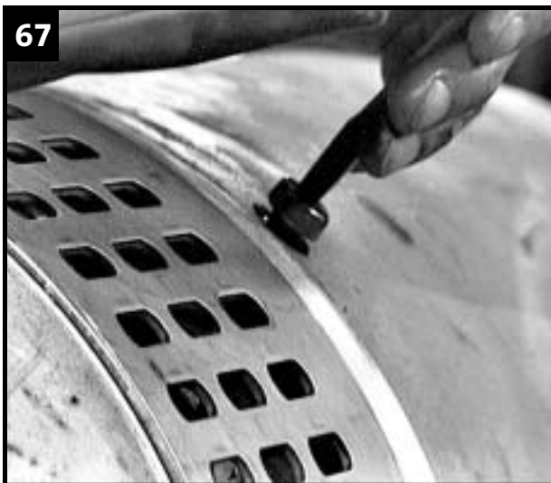
Fill oil chamber with one litre of Shell Ondina 15 oil and fit oil screw.
