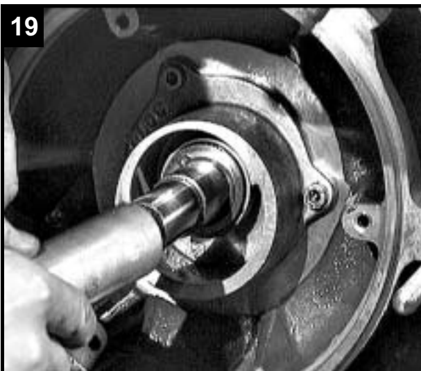
Press circlip into groove in shaft.
