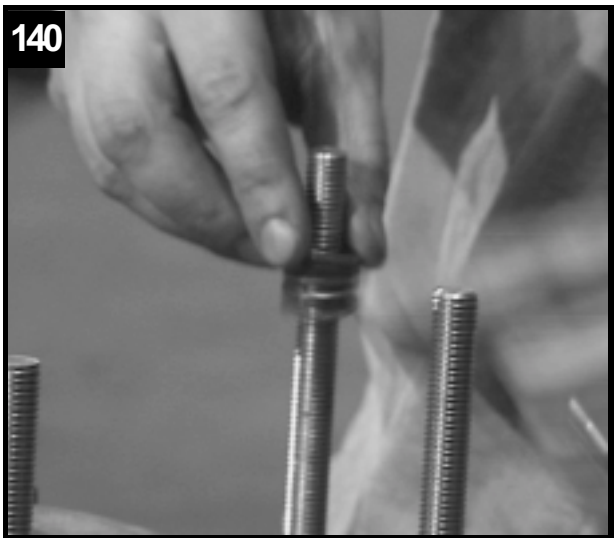
Fit four spacers on each staybolt.
