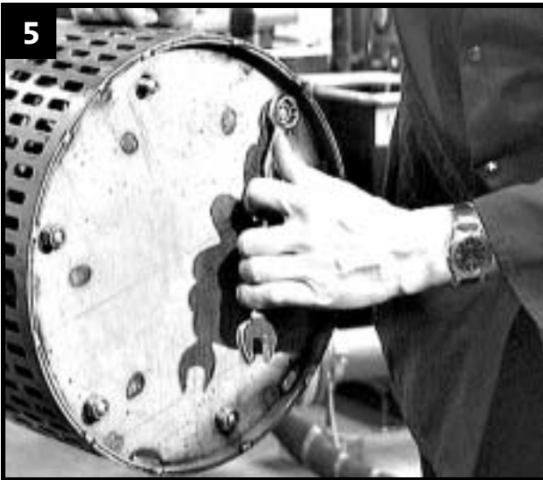
Remove nuts in strainer.
