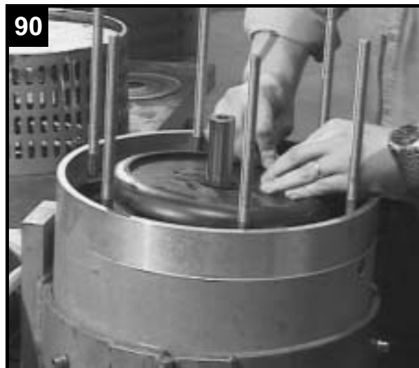
90 Press impeller disc to one side ...
