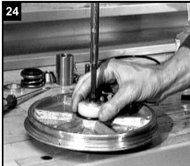
24 Tighten screw in tool until shaft seal part is in bottom position.
