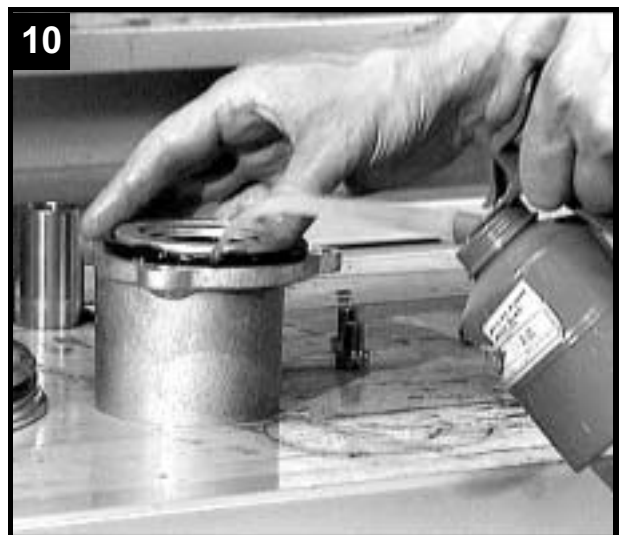
10 Fit O-ring on bearing cover and lubricate it.
