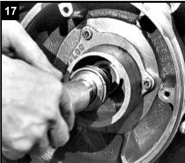
Press shaft seal and washer into position.
