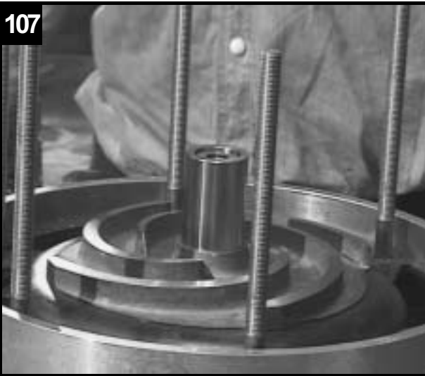
Fit temporary spacer.
