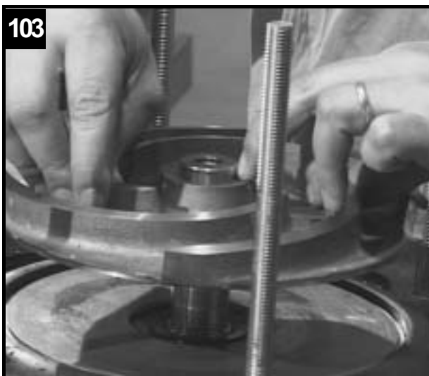
103 Remove impeller screw and impeller.
