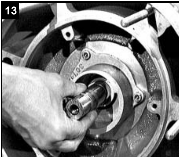
13 Fit protecting ring on shaft.
