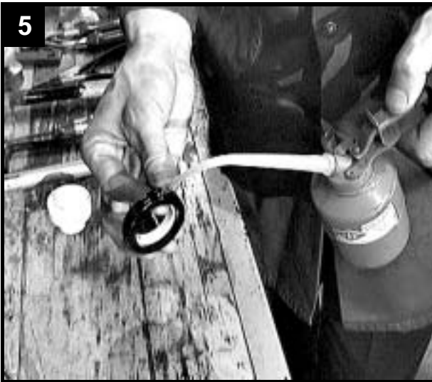
5 Lubricate rubber on stationary shaft seal unit.
