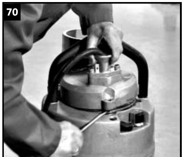
Lift off top cover carefully.
