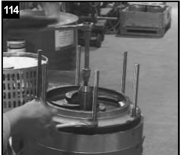
Fit and adjust nuts for minimum space between diffuser and impeller.
