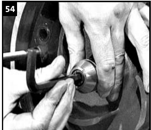
Fit impeller washer and screw.
