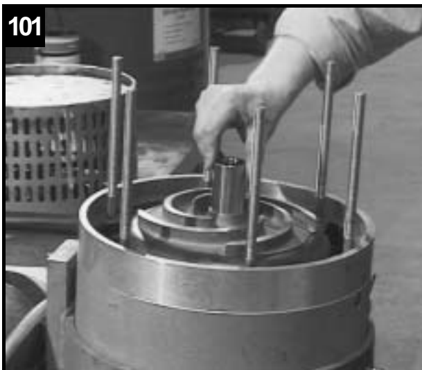
101 Fit temporary spacer.
