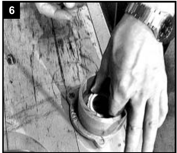
6 Place stationary shaft seal unit in bearing cover.
