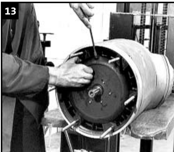
Loosen and remove impeller disc by means of a screw driver.
