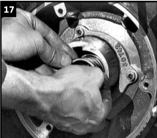
Remove rotating part of lower shaft seal.
