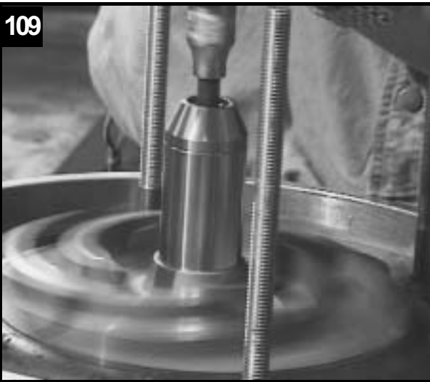
Tighten impeller screw.
