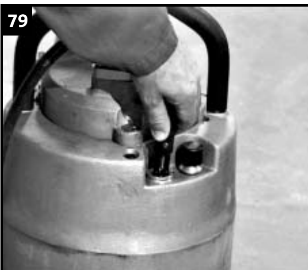
Fit electrode unit again.
