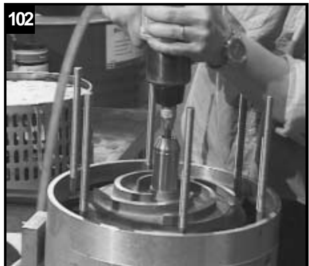
102 Fit and tighten impeller screw.
