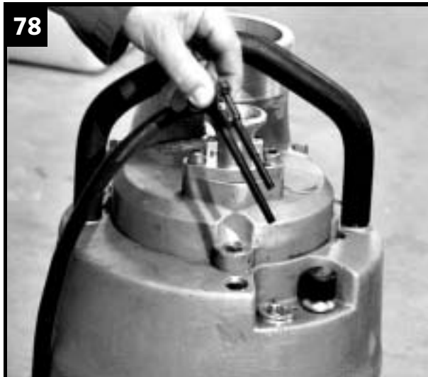
Clean electrodes for deposits.
