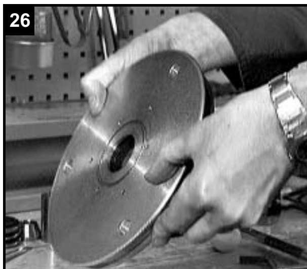
26 Inspect shaft seal unit for correct position.
