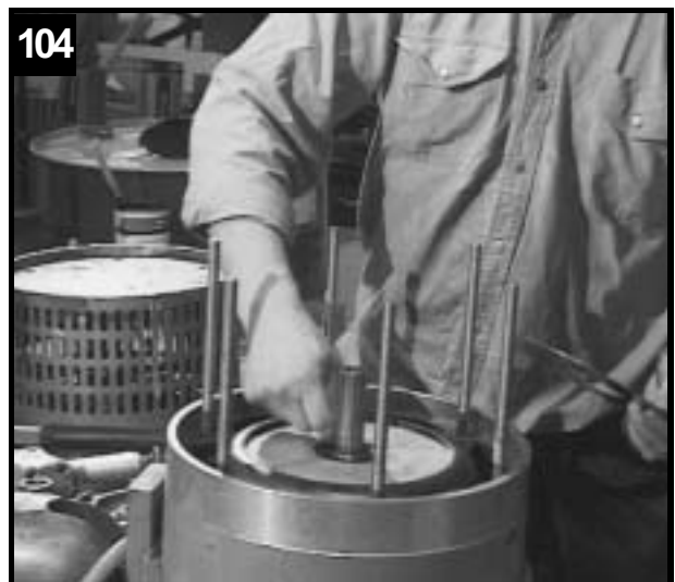
104 Remove impeller distance tools.
