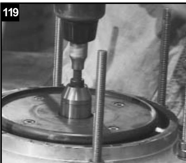
119 Remove impeller screw ...
