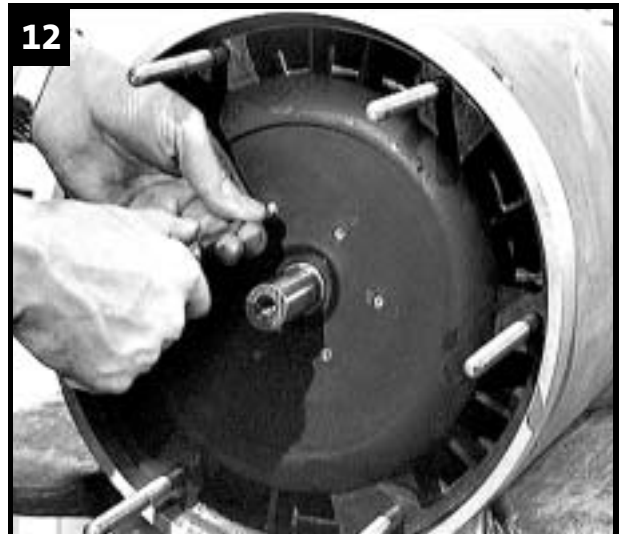
Remove screws in impeller disc.
