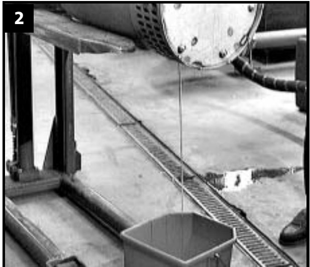
Drain off oil from chamber. - Beware of overpressure.
