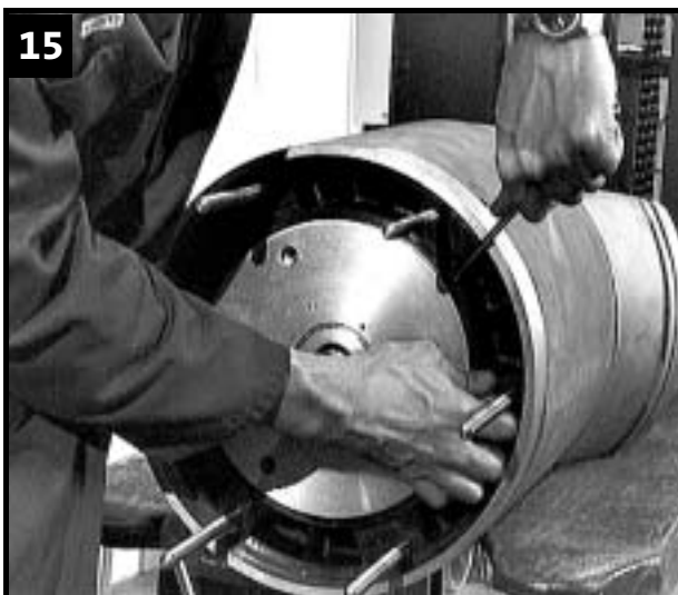
Loosen oil housing cover ....
