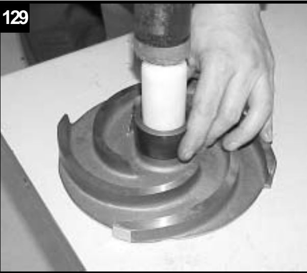
Position bushing in impeller.
