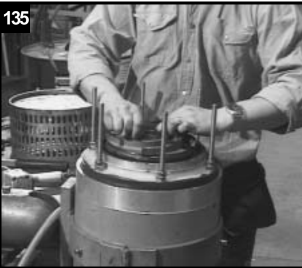
Fit second impeller again.
