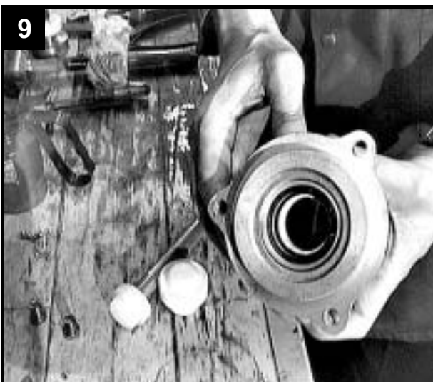
9 Check position of shaft seal unit.
