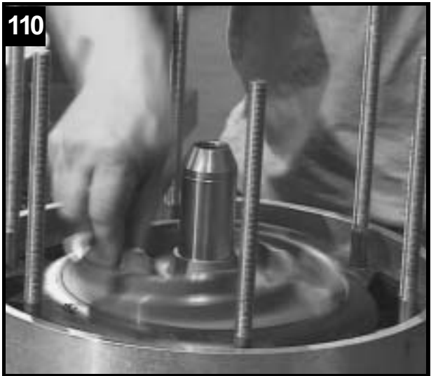
Test for free rotation.
