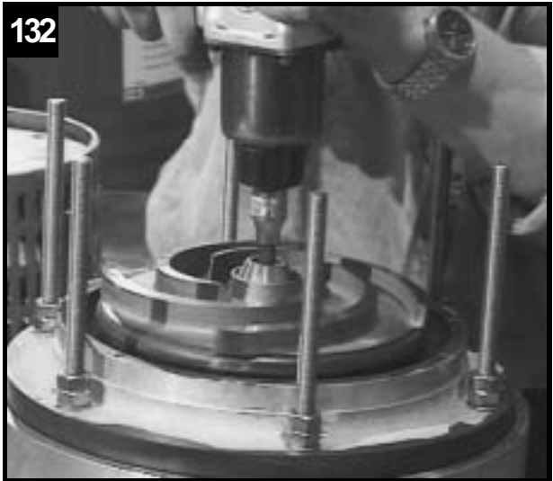
Tighten and loosen impeller screw.
