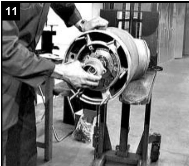
11 Fit bearing cover on motor housing.
