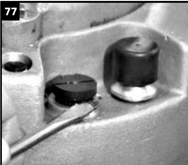
Lift up electrode unit.
