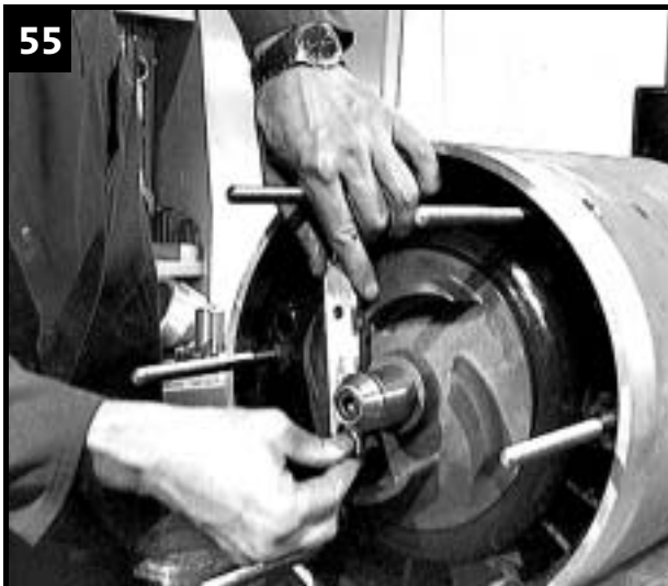
Use a tool to lock impeller.
