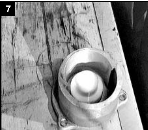
7 Place special tool on top of shaft seal unit ...
