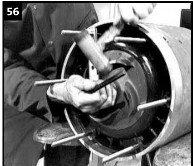
Tighten impeller screw.
