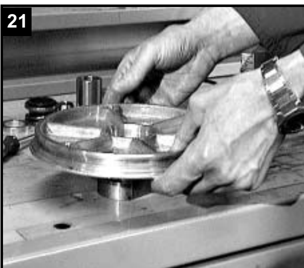
Place special tool under oil housing cover.
