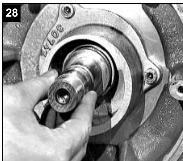
28 Fit protecting ring on shaft.
