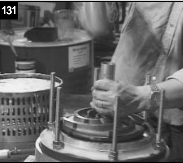
Tap split bushing into position.
