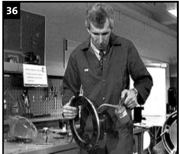
Lubricate rubber lining to ease assembly.
