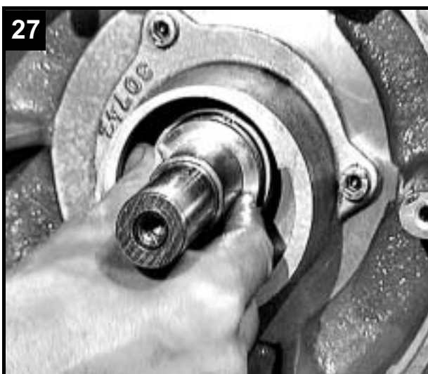
27 Fit washer for lower shaft seal.
