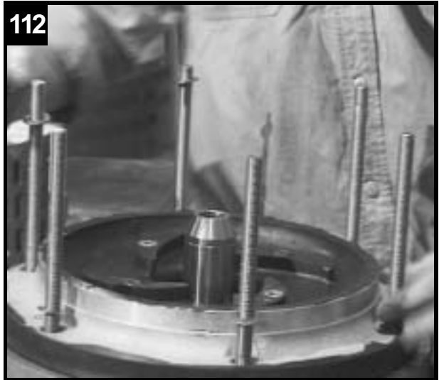
Fit washers on studs.
