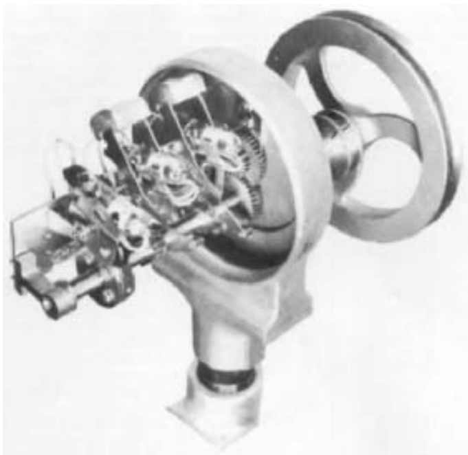
FIGURE 3 Mercury switches in liquid level sensor head are tripped by adjustable cams (Autocon Industries).
