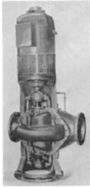
FIGURE 106 A vertical double-suction volute pump with a direct-mounted motor (Flowserve Corporation)
