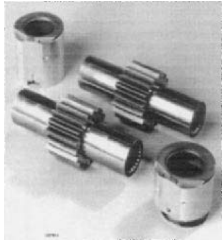
FIGURE 15 Spur gear pump gears and bearings (Courtesy Hamilton Sundstrand)
