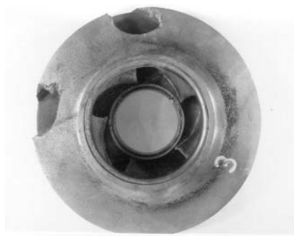
FIGURE 19 Overall view of a CF-3M impeller that has two corrosion-fatigue fractures in the front shroud wall
