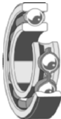
FIGURE 88 Single-row, deep-groove ball bearing (SKF USA, Inc.)
