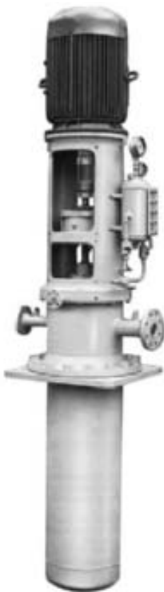
FIGURE 111 Vertical turbine can pump for condensate service (Flowserve Corporation)
