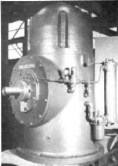
FIGURE 1 Spiral-bevel gear, right-angle vertical pump drive
