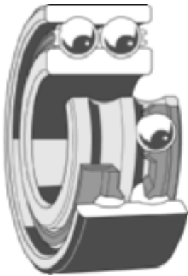
FIGURE 90 Double-row, angular-contact bearing (SKF USA, Inc.)
