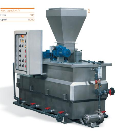
The Powder dilution plant is fitted with a stocking hopper and a volumetric endless screw, while the Emulsion dilution plant works thanks to a Plunger metering pump, dosing the Emulsion into a static mixer
